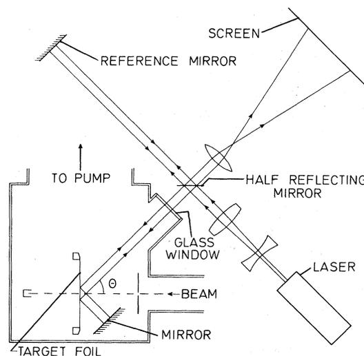
FIG. 2. Michelson interferometer arrangement for calibration and on-line control of the flatness of the target foil.
