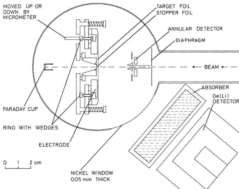
FIG. 1. Setup of the recoil-distance lifetime measurement.
