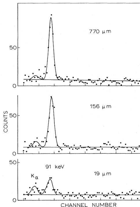
FIG. 3. Coincident  $\gamma$ -ray spectra as a function of distance. The drawn curves are the result of five Gaussian fits on a linear background.
