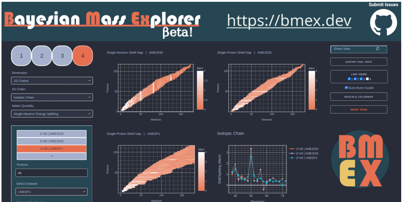
FIG. 8. Sample screenshot of the Bayesian Mass Explorer web interface in a configuration similar to what was used for the present investigation. The configuration and quantity of interest for each plot is accessed through the tab functionality on the left and additional data series can be added to the isotopic chains in the sidebar. The current view can be saved and shared using the “Share View” button on the right sidebar. Vector graphics in the PDF format can also be exported through the web interface for easy integration into documents.
