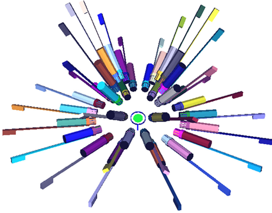
FIG. 5. MCNP version of the ELISA spectrometer. In the geometry, the sample holder, the ^{54}\text{Fe} disk, the 32 liquid organic scintillators, and their respective mounting are included.
