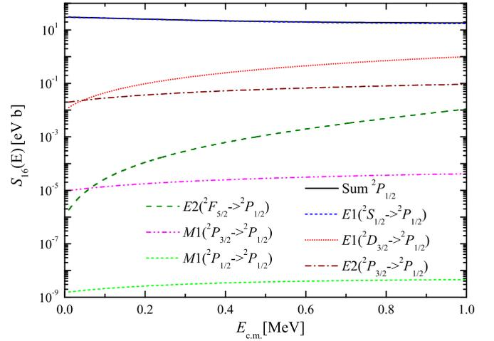
FIG. 5. Contributions of the  $E1$ ,  $E2$ , and  $M1$  transition operators to the astrophysical  $S$  factor from different initial scattering states to the final  ${}^7\text{Be}(1/2^-)$  excited bound state within the  $V_M$  potential model.
