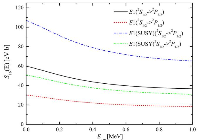
FIG. 3. Effect of the SUSY transformation of the  $S$ -wave potential on the  $E1$  astrophysical  $S$  factor within the potential model  $V_M$ .
