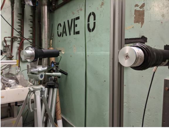
FIG. 9. Photo of the EJ-309 neutron scintillation detectors used in the time-of-flight experiment. Pictured here are the detectors positioned at 0^\circ and 18.2^\circ .
