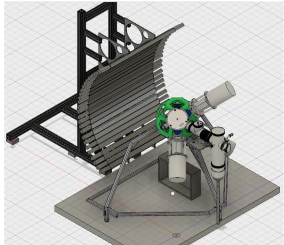
FIG. 1. Schematic drawing of experimental setup at IDS. The radioactive beam from ISOLDE was implanted on the tape at the center of the setup. The  $\beta$ -delayed  $\gamma$  rays from  $^{133}\text{In}$  were detected by four HPGe clover detectors at backward angles relative to the beam direction. The INDiE array was placed on the other side to measure neutron spectroscopy following the  $^{133}\text{In}$  decay.
