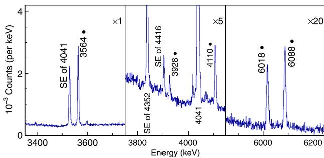
FIG. 4. Portion of  $\gamma$ -ray spectra measured in coincidence with the ground-state decay of  $^{133}\text{In}$ . The candidate  $\gamma$  deexcitations from the  $^{133}\text{Sn}$  neutron-unbound states are marked by “●” to be distinguished from the  $\gamma$  decays in  $^{132}\text{Sn}$ . SE stands for “single-escape” peak. See text for details.
