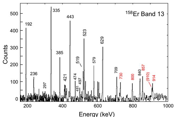
FIG. 18. Sample spectrum from the thick-target data for band 13 in  $^{158}\text{Er}$  (a triple gate between the 755 keV decay, transitions in band 13 and transitions in band 4; see text for details). The labeling convention used in Fig. 7 is adopted.
