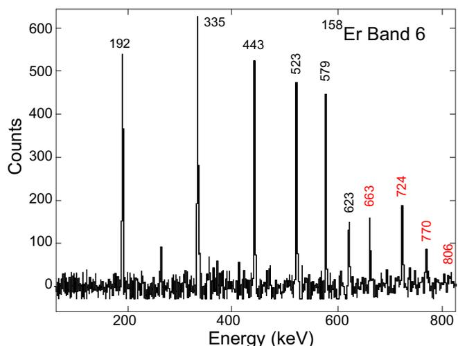
FIG. 12. Sample spectrum from the thick-target data for band 6 in  $^{158}\text{Er}$ , selected to show the new transitions. Sum of two triple gates, one on the 608, 602, and 623, the other on the 608, 602, and 663 keV  $\gamma$  rays. The labeling convention used in Fig. 7 is adopted.
