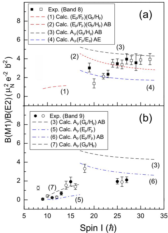
FIG. 22. Measured  $B(M1)/B(E2)$  ratios of reduced transition probabilities as a function of spin for bands 8 (top panel) and 9 (bottom panel) in  $^{158}\text{Er}$ . Open (filled) symbols denote the signatures  $\alpha = 0$  (1). The configurations for the theoretical calculations are given in the boxes.
