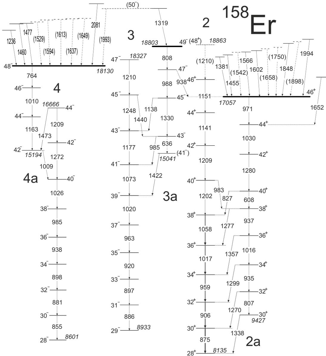
FIG. 5. High-spin section of the  $^{158}\text{Er}$  level scheme displaying bands 2, 3, and 4 from spin  $28\hbar$ . Band-terminating states at  $46^+$ ,  $48^-$ , and  $49^-$  are indicated by thickened lines. The same labeling convention as in Fig. 3 is employed, with additional labels, 2a, 3a, and 4a, to distinguish the terminating sequences; see discussion.
