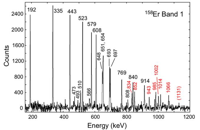
FIG. 7. Summed spectrum representative of band 1 in  $^{158}\text{Er}$  (in coincidence with three of the transitions in this band; see text for details) from the thick-target experiment. The energies of the new transitions are highlighted in red, and previously published ones are in black. Tentative transitions are given within parentheses.
