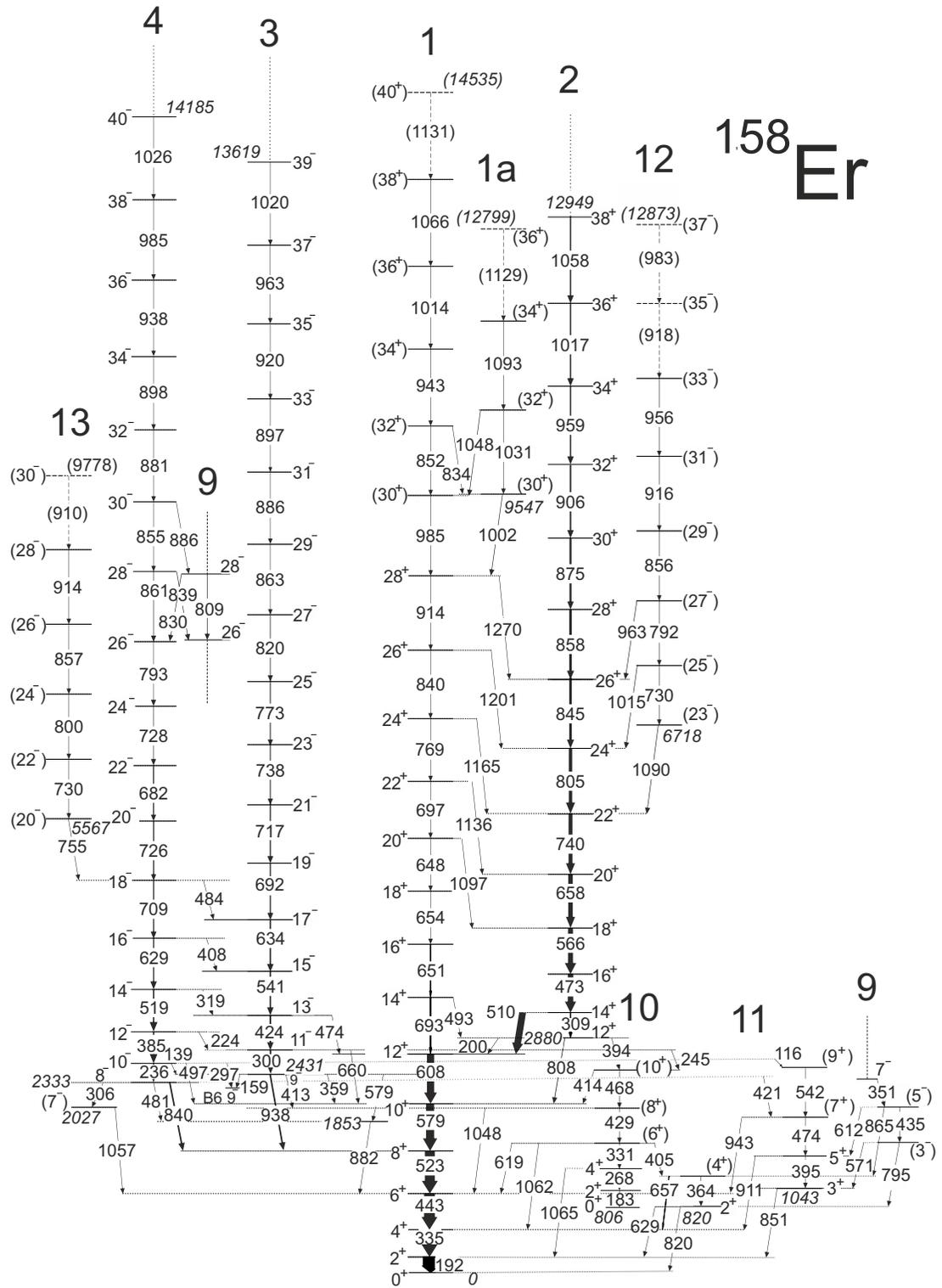
FIG. 3. Partial level scheme of  $^{158}\text{Er}$  showing bands 1 to 4 and 10 to 13 below spin  $40\hbar$ . Energies are given in keV, tentative transitions and levels are indicated by dashed lines, and tentative spins, parities, and  $\gamma$ -ray energies are given within parentheses. The less energetically favored branch in band 1 above  $28^+$  is labeled 1a. Extension of bands 2–4 to higher spin (Fig. 5) and connections to band 9 (Fig. 4) are indicated.
