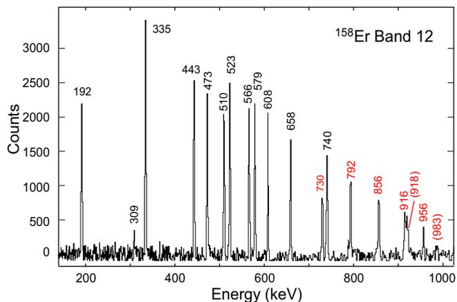
FIG. 17. Sample spectrum from the thick-target data for band 12 in  $^{158}\text{Er}$  (in coincidence with the 1090 keV decay, yrast band transitions and transitions in band 12; see text for details). The labeling convention used in Fig. 7 is adopted.
