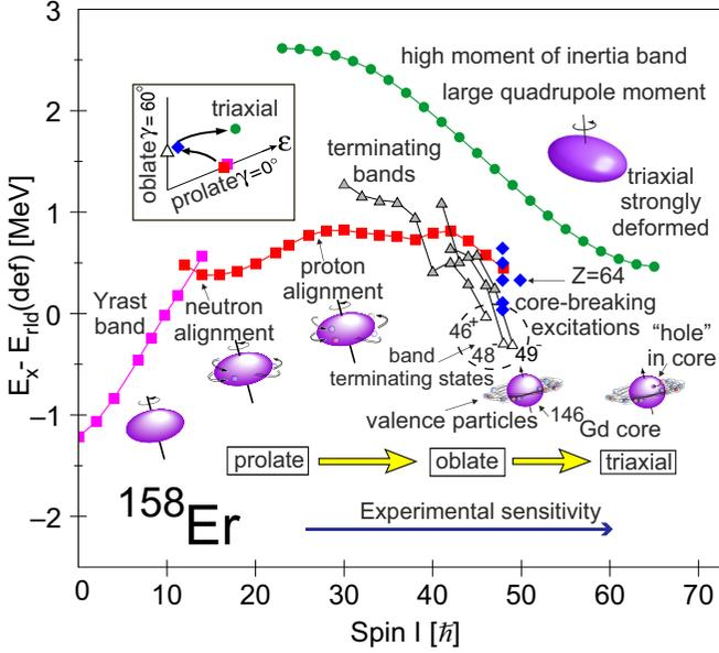
FIG. 1. The evolution of nuclear structure in  $^{158}\text{Er}$  as a function of spin and excitation energy. The inset illustrates the changing shape of  $^{158}\text{Er}$  with increasing spin within the standard  $(\epsilon, \gamma)$  deformation plane. Excitation energies are plotted relative to a deformed rotating liquid drop reference [13]; see also [14]. This figure is adapted and updated from Ref. [15].
