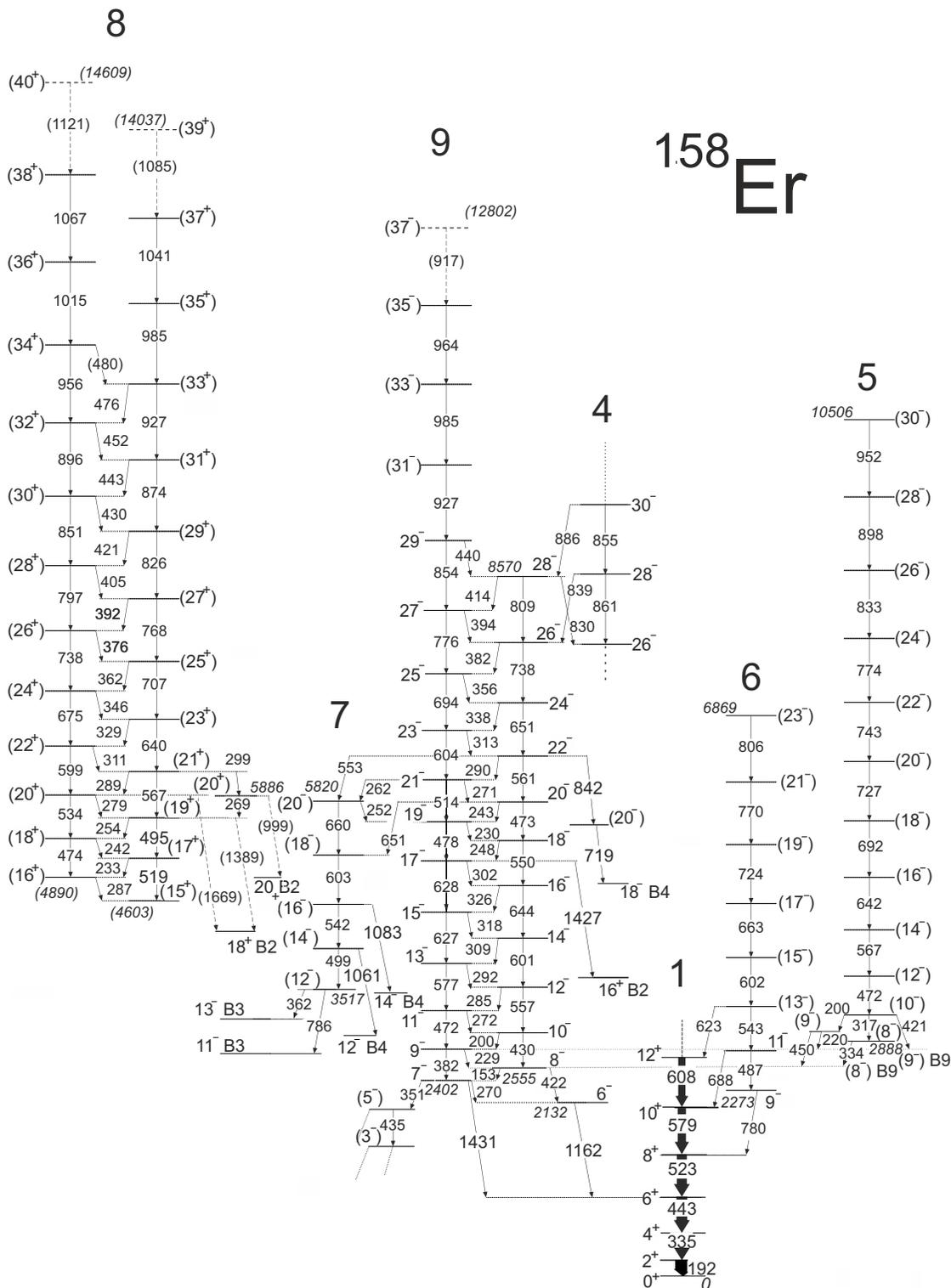
FIG. 4. Partial level scheme of  $^{158}\text{Er}$  showing bands 5 to 9 and the low lying states in band 1. Connections to states in bands 2, 3, and 4 are indicated. The decay from band 9 via the 351 and 435 transitions are shown in Fig. 3. The same labeling convention as in Fig. 3 is employed.
