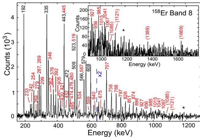
FIG. 14. Sample spectrum from the thick-target data for band 8 in  $^{158}\text{Er}$  (in coincidence with the 311 and the 329 keV transitions in this band). In order to highlight the high-energy weak transitions in this band, the portion of the spectrum above 900 keV has been magnified (times 2) and an inset of the same spectrum for the 900–1800 keV energy range is presented. The labeling convention used in Fig. 7 is adopted.
