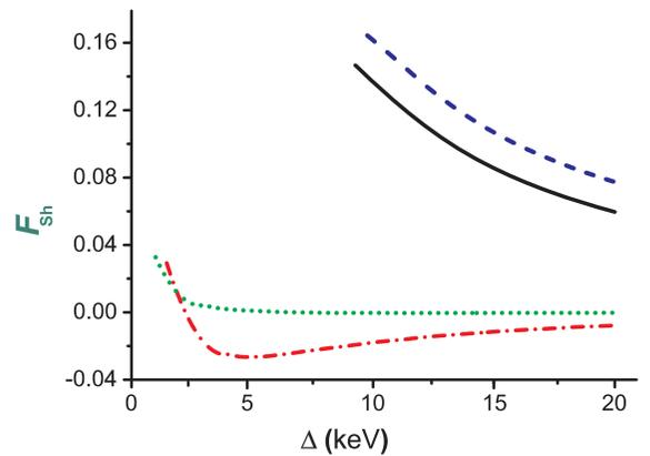
FIG. 5. Comparison of shell contributions to the shake amplitude as a function of the orbital angular momentum. Matrix elements  $F_{\text{sh}}$  for the  $2s$  subshell (dashed line),  $2p_{1/2}$  subshell (solid curve),  $3d_{3/2}$  (dash-dotted line), and  $4f_{5/2}$  (dotted line) subshells of  $^{164}\text{Dy}$  atom.
