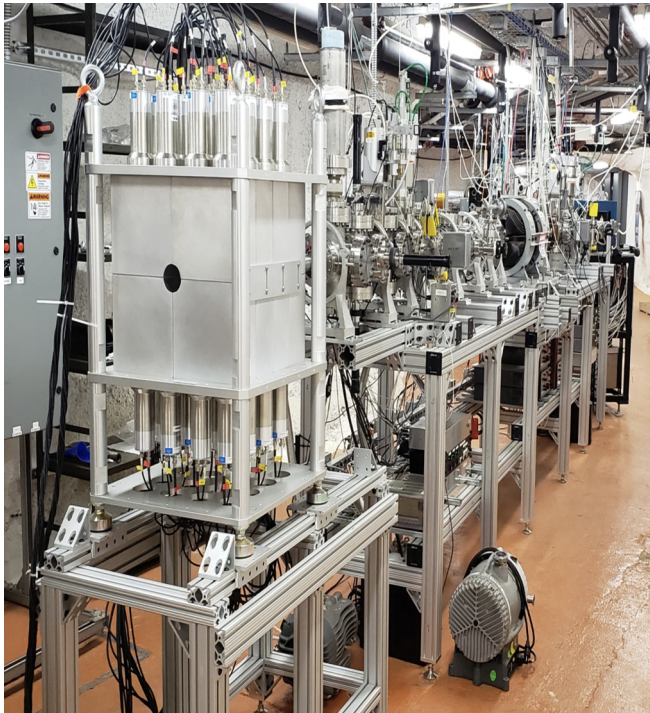
FIG. 3. Experimental setup showing HECTOR placed at the end of the beamline at the CASPAR underground laboratory. The target is placed at the center of the detector cube.
