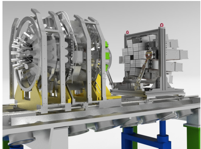
FIG. 1. Rendering of the INDRA-FAZIA mechanical coupling, with INDRA on the left side and FAZIA on the right side. The target holder, not visible in the picture, is located inside the INDRA apparatus.
