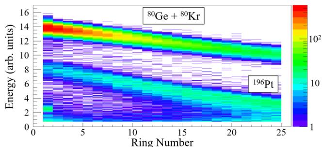
FIG. 1. The energy deposited in the downstream silicon detector. The scattered projectiles and recoiling  $^{196}\text{Pt}$  nuclei are clearly visible and distinguishable. It is also clear there is no separation between the  $^{80}\text{Ge}$  nuclei and the  $^{80}\text{Kr}$  contamination.
