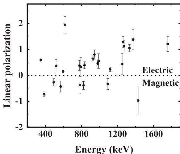
FIG. 3. The linear polarizations for some observed transitions in  $^{62}\text{Cu}$ . In general, a positive value corresponds to an electric transition, and a negative value indicates a magnetic transition.
