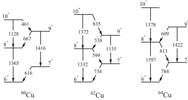
FIG. 4. Comparison of the negative-parity structures built on the  $6^-$  level in  $^{60}\text{Cu}$  [18],  $^{62}\text{Cu}$ , and  $^{64}\text{Cu}$  [17].
