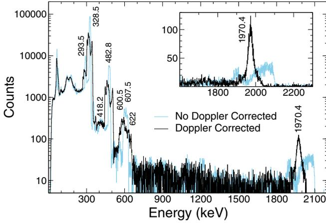
FIG. 2. Doppler (black) and non-Doppler (blue) corrected  $\gamma$ -ray energy spectra in log  $\gamma$  scale for the  $^{194}\text{Pt}(^{36}\text{Ar}, ^{36}\text{Ar}^*)^{194}\text{Pt}^*$  reaction at 134.2 MeV. The inset shows the 1970.4-keV peaks in  $^{36}\text{Ar}$  with and without Doppler correction in a linear scale.
