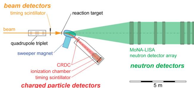
FIG. 1. Schematic layout of the  $^{33}\text{Mg}(-2p)$  experiment. See text for details.
