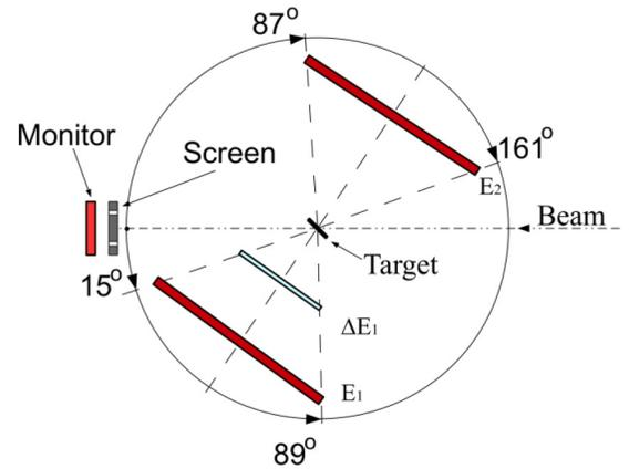
FIG. 1. Sketch of the detection system for the measurements, composed by one  $\Delta E$ - $E$  telescope, placed at forward angles, and an  $E$ -detector at backward angles. The  $E$ -detectors are  $128 \times 128$  DSSSD and the  $\Delta E$  is a  $16 \times 16$  thin DSSSD. A third DSSSD (monitor) was placed at  $0^\circ$  to monitor the beam axis.
