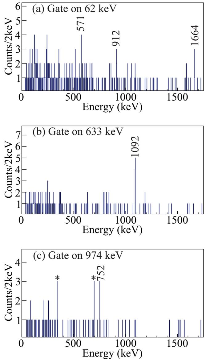
FIG. 2.  $\gamma$ - $\gamma$  coincidence spectra for (a) the 62-, (b) the 633-, and (c) the 974-keV transition in  $^{137}\text{Te}$ . Coincident transitions are indicated with their energies and contaminants are labeled with asterisks (\*).
