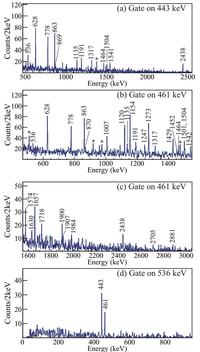
FIG. 5.  $\gamma$ - $\gamma$  coincidence spectra with gate on (a) the 443-keV, (b),(c) the 461-keV, and (d) the 536-keV transition. Coincident transitions are indicated with their energies and contaminants are labeled with asterisks (\*).
