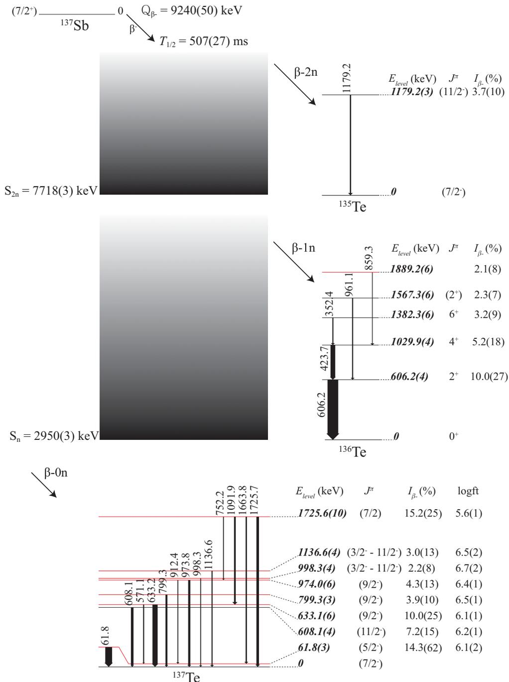
FIG. 3.  $\beta$ -decay scheme of  $^{137}\text{Sb}$ . The half-life of the ground state of  $^{137}\text{Sb}$  is based on the present work. The  $Q_{\beta}$ - and neutron separation energies ( $S_n$ ,  $S_{2n}$ ) are taken from Ref. [23]. Level information such as excitation energies, spin-parities,  $\beta$ -branching ratios, and log  $ft$  values are represented. Excited states newly established in the present work are represented in red.
