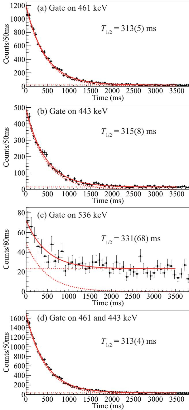
FIG. 6. Half-life measurements of the ground state of  $^{138}\text{Sb}$ . Red solid lines indicate the fit results with a single-component exponential decay curve (red-dashed lines) and a constant background (red dashed-dotted lines).
