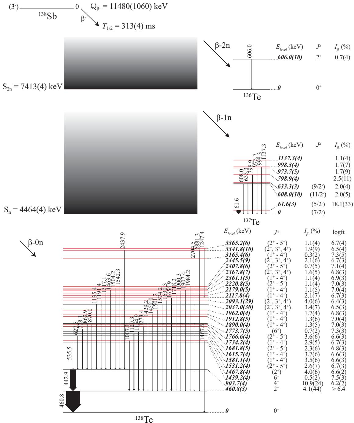
FIG. 7.  $\beta$ -decay scheme of  $^{138}\text{Sb}$ . The half-life of the ground state of  $^{138}\text{Sb}$  is based on the present work. The  $Q_{\beta^-}$ - and neutron separation energies ( $S_n$ ,  $S_{2n}$ ) are taken from Ref. [23]. Level information such as excitation energies, proposed spin-parities,  $\beta$ -branching ratios, and log  $ft$  values are represented. Newly assigned excited states from the present work are represented in red.
