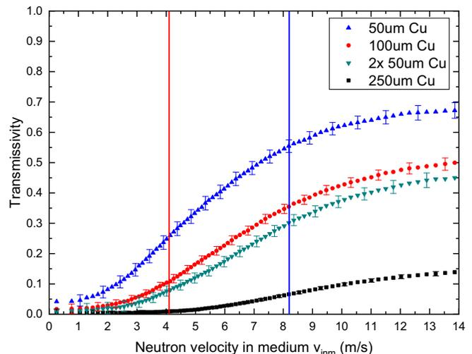
FIG. 1. Measured transmissivity of Cu foils for UCNs plotted over UCN velocity. The in-medium velocity of 4.1 m/s (equivalent to 7 m/s out of medium) is marked with a vertical red line. The vertical blue line marks 8.2 m/s (equivalent to 10 m/s out of medium). For data treatment, a sliding average of 16 time bins was used. The error bars account for this. To improve legibility, only every fourth error bar is shown.
