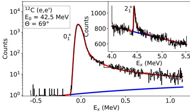
FIG. 1. Elastic electron-scattering spectrum taken at a beam energy of 42.5 MeV and a scattering angle of 69°. The inset shows the excitation of the  $2_1^+$  state. The light gray (red) lines display a fit using Eq. (1) and the dark gray (blue) lines a linear background.
