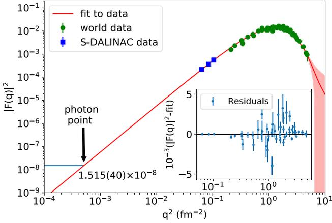
FIG. 3. Experimental form factor of the transition to the  $2_1^+$  state in  $^{12}\text{C}$  after the DWBA corrections described in the text. Data from the present work are shown as (blue) squares and previous measurements [35–38] as (green) circles. Most of the error bars are smaller than the displayed data points. The (red) band shows a fit of Eq. (3) with a  $1\sigma$  uncertainty. The arrow indicates the photon point. The inset shows the scattering of the residuals around the fit.
