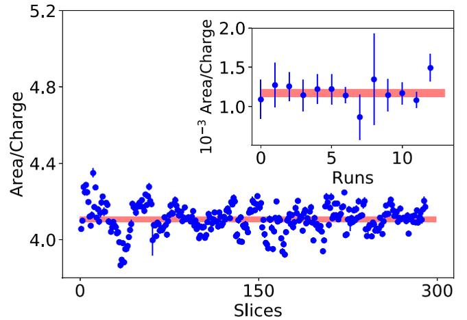
FIG. 2. Area/charge ratios for slices of the elastic line measurements at 69° (circles) and uncertainty-weighted average band. The inset shows corresponding values for the excitation of the  $2_1^+$  state.
