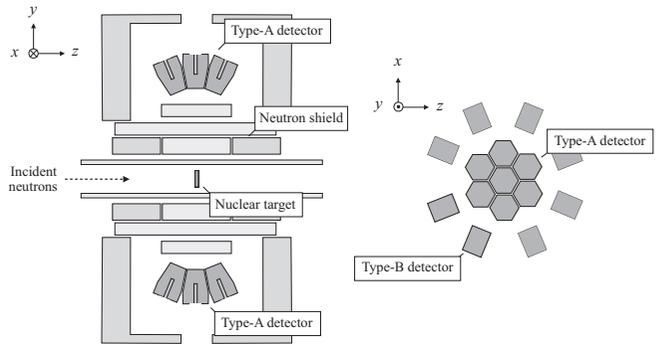
FIG. 2. Germanium detector assembly. The left figure is a sectional view and the right figure is a top view.
