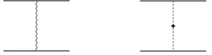
FIG. 11. Long-range contributions to the CIB NN potential. The wavy line represents a photon and the star denotes an insertion of the electromagnetic pion-mass splitting. Other symbols are as in Fig. 1.
