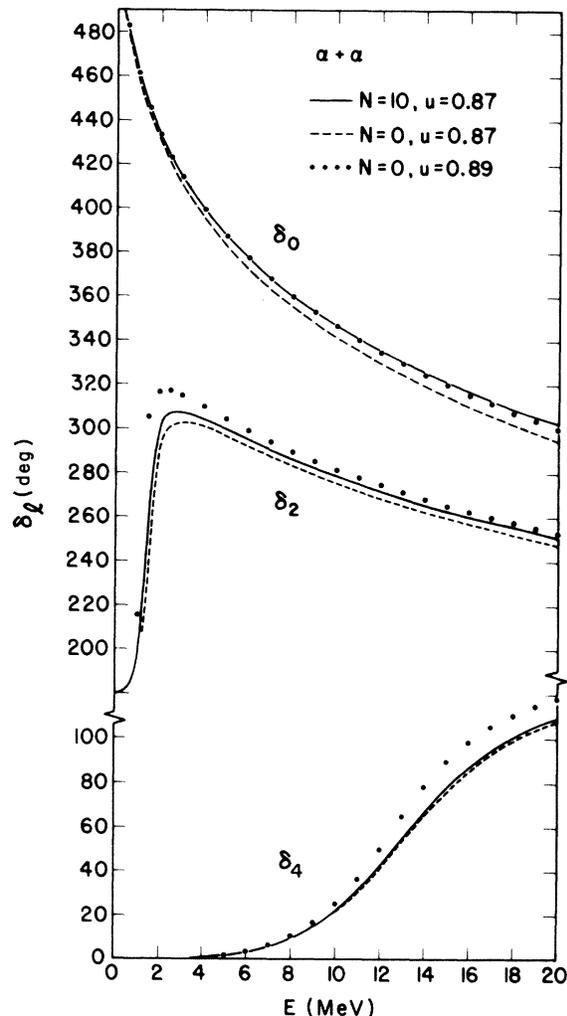
FIG. 2.  $\alpha + \alpha$  phase shifts as a function of energy for  $l=0, 2,$  and  $4$ . The solid curves show phases calculated using ten distortion functions of configuration I and  $u = 0.87$ . The dashed curves and the solid dots show phases calculated using no distortion and  $u=0.87$  and  $0.89$ , respectively.
