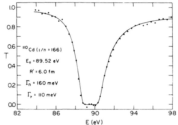
FIG. 2. Result of a shape fit to the transmission data of the  $^{110}\text{Cd}$  separated isotope ( $1/n = 166$  b/atom) for the strong level at 89.52 eV with the indicated parameters. The analysis uses a Breit-Wigner single level formula, including the Doppler effect and the  $(E)^{1/2}$  variation of  $\Gamma_n$ . The interference asymmetry, permits an evaluation of  $R'$ , giving  $R' = 6.0$  fm for this level.
