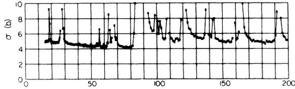
FIG. 1. The between level total cross section vs energy for natural Cd to 200 eV with sample thickness  $1/n = 5.36$  b/atom. Each plotted point represents a many channel average satisfying the requirements that  $(T_{\max} - T_{\min}) < 0.1$  within the average group, and that  $\sigma < 10$  b where  $\sigma = -(1/n) \ln \langle T \rangle$  (or else the average is not used). A line connecting two neighboring points means that no excluded set of channels comes between them.
