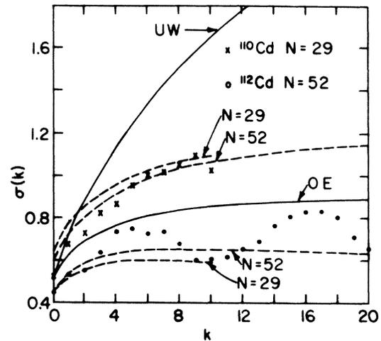
FIG. 8. Comparison of  $\sigma(k)$  values for our selected  $s$  level sets for  $^{110}\text{Cd}$  to 5 keV and  $^{112}\text{Cd}$  to 7 keV with Monte Carlo results for OE and UW theories.  $\sigma(k)$  is the standard deviation from the mean for the spacings of levels having  $k$  levels between  $(\ln \text{ units of } \langle D_0 \rangle)$ . The dashed curves give the 10 and 90% confidence limits for OE for the two isotopes.
