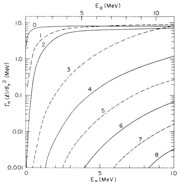
FIG. 6. Plot of  $\Gamma_n/\theta_n^2$  in MeV versus the neutron decay energy  $E_n$  as a function of  $l_n$  for the neutron decay of unbound states of  ${}^{15}\text{C}$ . See Sec. III B for details of the penetrability calculation. Also shown is an excitation energy scale in  ${}^{15}\text{C}$  assuming decay to the  ${}^{14}\text{C}$  ground state. Values of  $R = 4.95$  fm and  $\gamma_n = 2.73$  MeV were used for the radius and Wigner limit, respectively, in the calculation.
