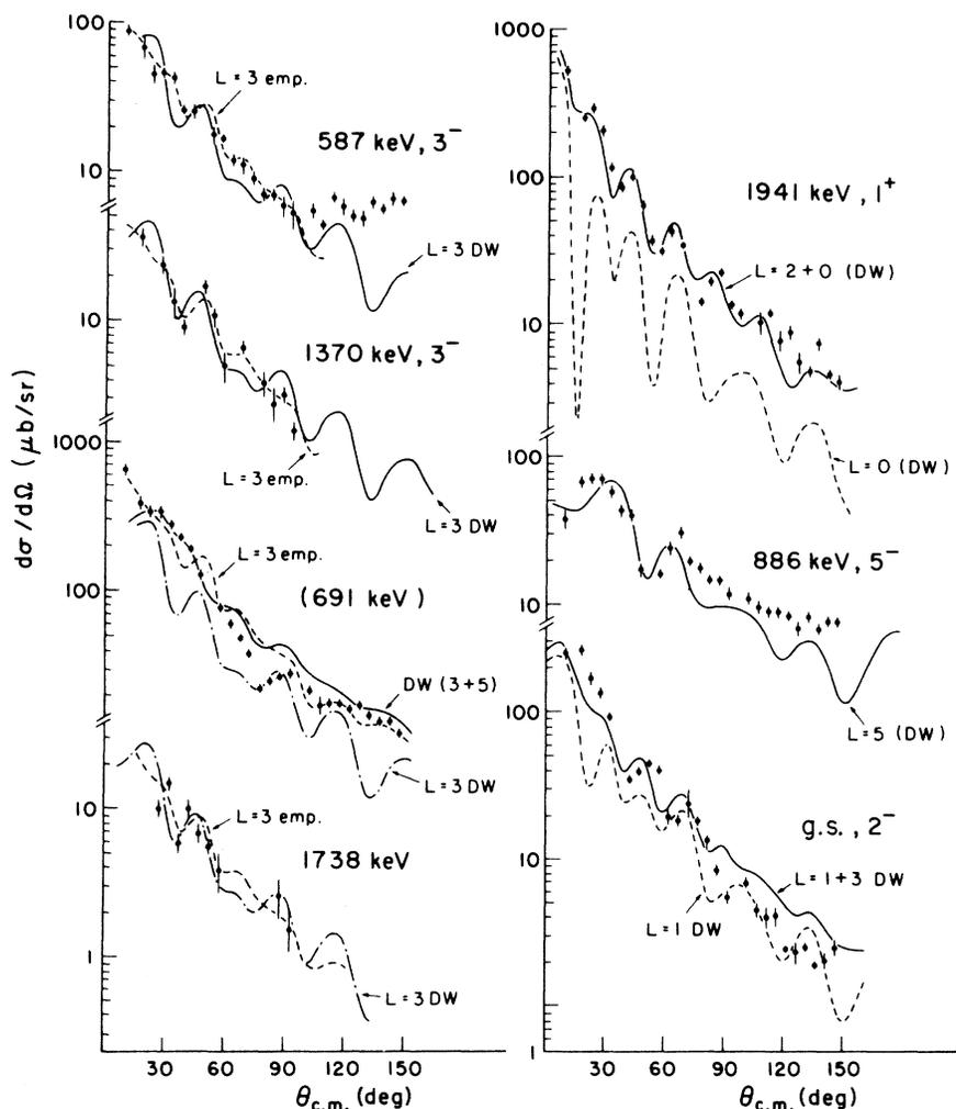
FIG. 4. Experimental  $^{48}\text{Ca}(d, \alpha)^{46}\text{K}$  angular distributions at  $E_d = 17$  MeV compared with DWBA calculations and empirical  $L = 3$  curves. For DWBA curves which are the sum of two  $L$  transfers the dominant contributor is also shown separately. Experimental error bars include statistics, random monitoring errors, and estimated errors due to background subtraction (in quadrature).
