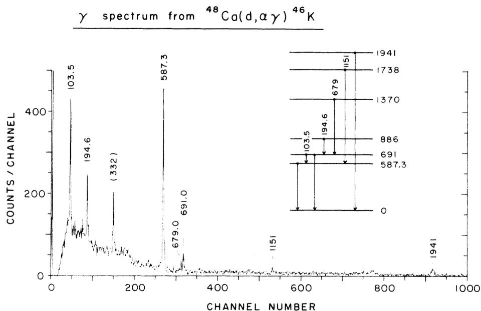
FIG. 1. Spectrum of all  $\gamma$  rays in fast coincidence with 4–8 MeV  $\alpha$ 's from the  $^{48}\text{Ca}(d, \alpha\gamma)^{46}\text{K}$  reaction at  $E_d = 7$  MeV. The insert shows the  $\gamma$  decay spectrum deduced from energy balance considerations and stripping of the two-dimensional  $E_\alpha - E_\gamma$  data set. The 332 keV transition stems from the  $^{40}\text{Ca}$  target impurity (see text).
