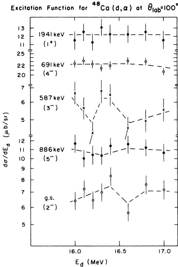
FIG. 3. Semilog plot of  $d\sigma/dE_d$  for  $^{48}\text{Ca}(d,\alpha)$  as a function of deuteron energy. The angle of observation was  $\theta_{\text{lab}}=100^\circ$ . A similar behavior was seen at  $\theta_{\text{lab}}=90^\circ$ . Fluctuations were significantly smaller at forward angles (i.e., inside statistics), except for the weak 1.738 MeV level (not shown).
