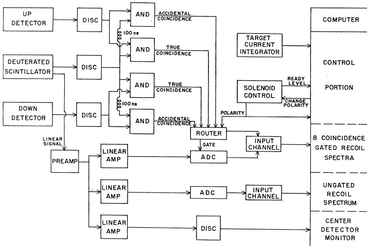
FIG. 1. Electronics diagram showing the fast-coincidence circuitry and the linear-signal analysis.
