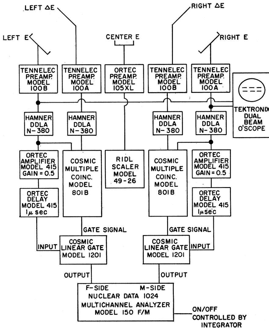
FIG. 2. The detector arrangement and block diagram of the electronics used in the polarization measurements.
