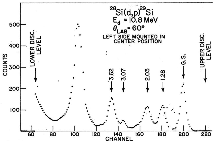
FIG. 3. A typical spectrum from the reaction  $^{28}\text{Si}(d,p)^{29}\text{Si}$  with a side-counter telescope mounted in the center position of the polarimeter. Discriminator settings and groups corresponding to excited states of  $^{29}\text{Si}$  are indicated by the arrows.
