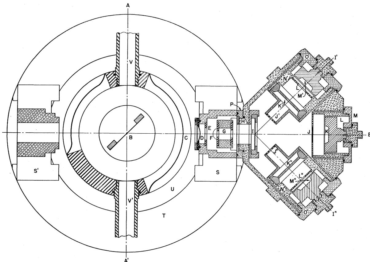
FIG. 1. A cross section through the median plane of the scattering-chamber-polarimeter assembly used to measure the polarizations of the reaction protons. Letter designations are explained in the text.
