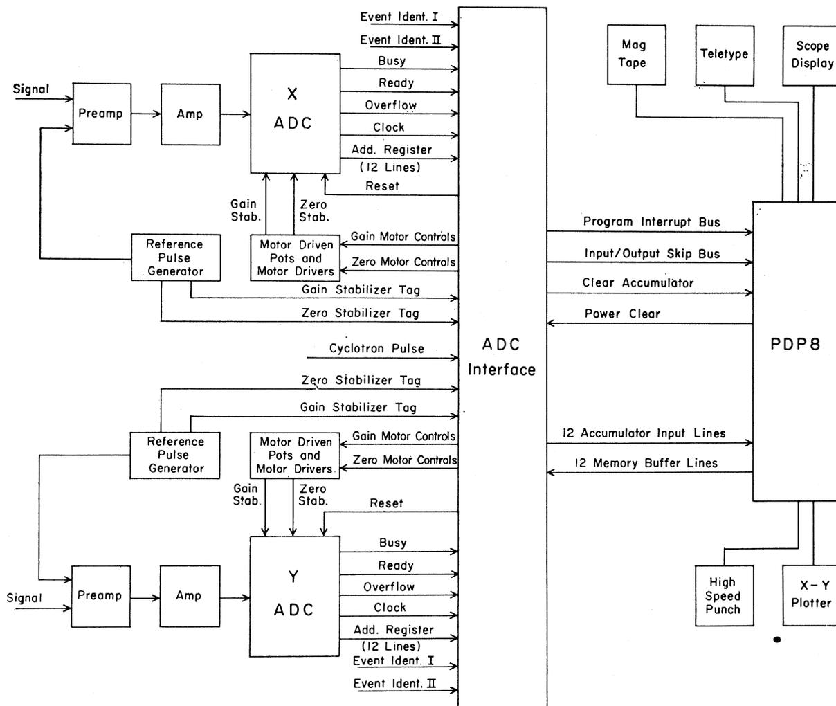
FIG. 5. Block diagram of interface to the PDP-8.
