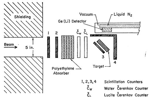
FIG. 2. Schematic diagram of beam telescope and Ge(Li) detector placement.
