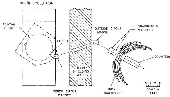
FIG. 1. Floor plan of the experimental arrangement.
