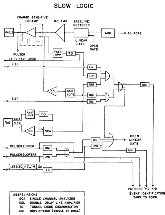
Fig. 4. Block diagram of the "slow logic": the detector circuitry, beam-detector coincidence logic, NaI(Tl)-Ge(Li) coincidence logic, and stabilization logic.
