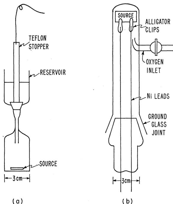
FIG. 2. (a) Apparatus for preparation of Nb (fluoride complex).
