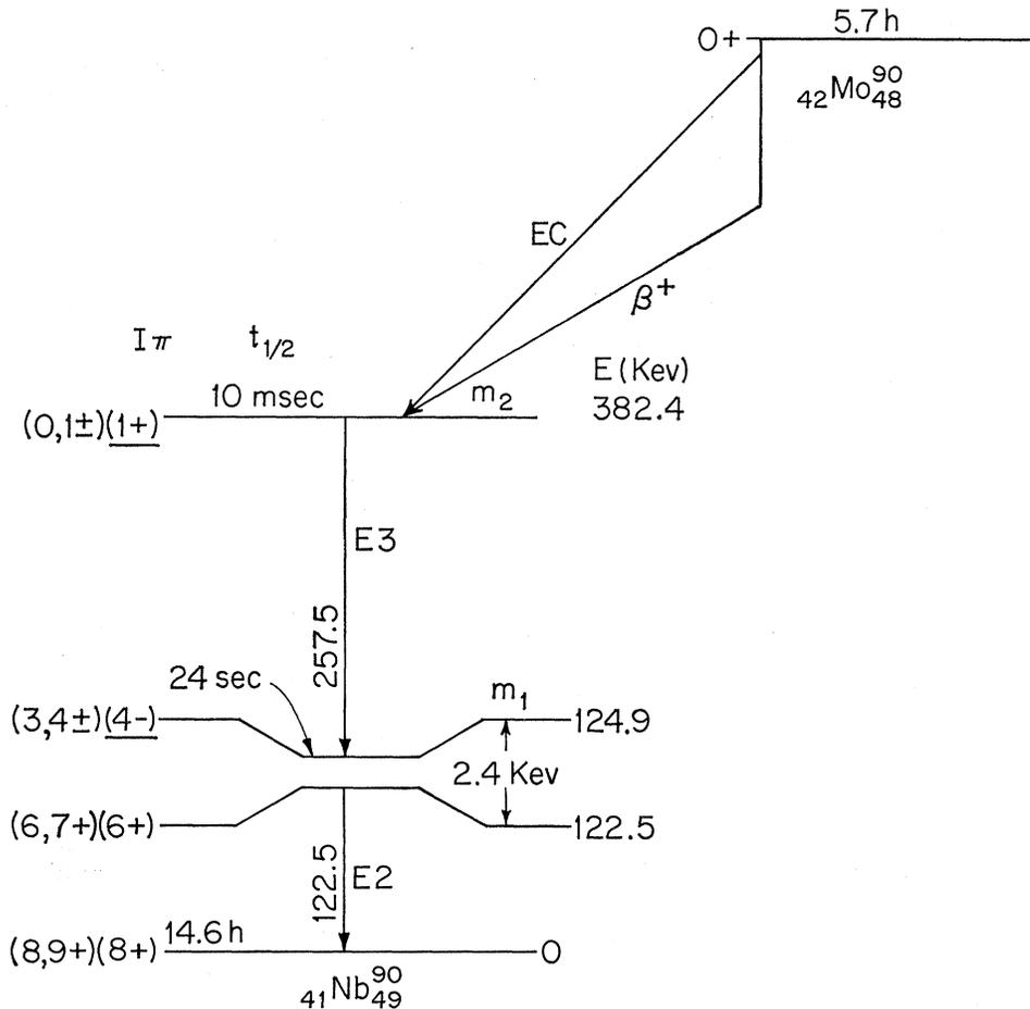
FIG. 1. Partial decay scheme of Mo<sup>90</sup> as proposed by Cooper *et al.* (Ref. 2). The first metastable state (Nb<sup>90m</sup>) at 124.9 keV is indicated by  $m_1$  and the second metastable state (Nb<sup>90m2</sup>) at 382.4 keV by  $m_2$ .
