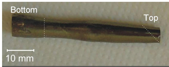
FIG. 20. The single crystal [50] of \text{Ce}(\text{Fe}_{0.76}\text{Ru}_{0.24})_2\text{Ge}_2 used for all single-crystal neutron scattering experiments. The part labeled “bottom” exhibited long-range order (see Fig. 6) and was part of the first HB3 experiments, subsequently masked with Gd paint for follow-up HB3 experiments, and cut off in later experiments (DCS, TRIAX, BT7). The part labeled “top” was cut off and used in specific heat, susceptibility, and resistivity measurements.
