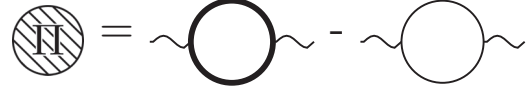
FIG. 5. Self-consistent equations for the self-energy and the polarization. Note that the bold lines on the right-hand sides also include the self-energy and the polarization.
