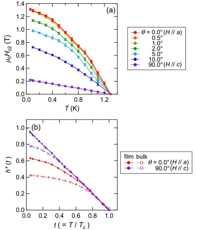
FIG. 3. Superconducting phase diagram in the crossover region. (a)  $H$ - $T$  phase diagram of superconductivity in the  $\text{Sr}_2\text{RuO}_4$  film at various field angles between  $\theta = 0^\circ$  and  $90^\circ$ . (b) Temperature dependence of the normalized upper critical field  $h^*(t)$  defined as  $h^*(t) = -H_{c2}(t) / (dH_{c2}/dt)|_{t=1}$  ( $t = T/T_c$ ), compared to the bulk one [13].
