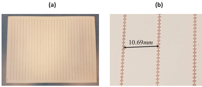
FIG. 4. (a) The fabricated MG prototype and (b) zoom-in on three lateral periods of the MG.
