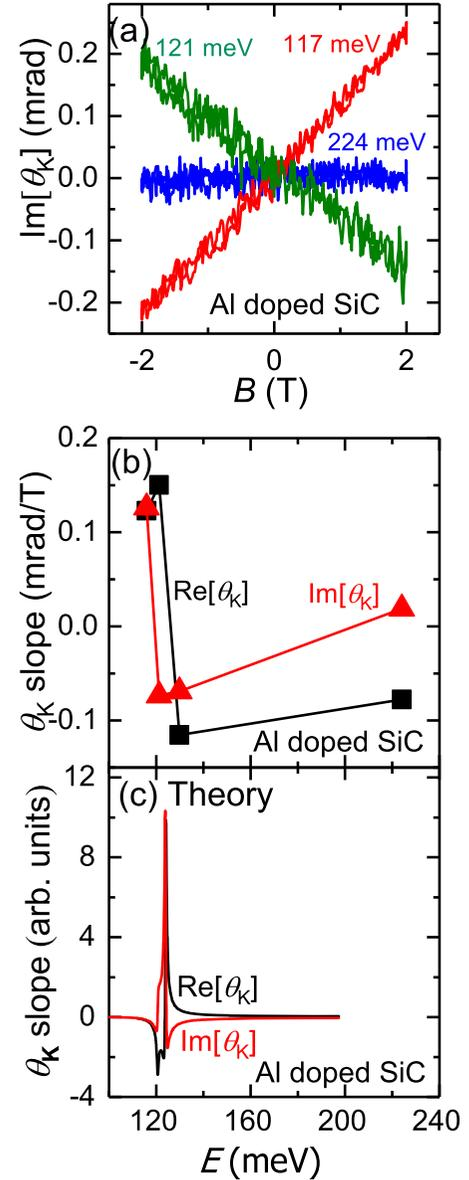
FIG. 3. (a). Magnetic field dependence of  $\text{Im}[\theta_K]$  for Al-doped 6H-SiC measured at 117-, 121-, and 224-meV photon energy. (b) Energy dependence of the measured slope. (c) Calculated Kerr angle line shape for bulk Al-doped 6H-SiC.
