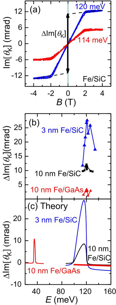
FIG. 2. (a) Magnetic field dependence of  $\text{Im}[\theta_K]$  for Fe film on SiC, measured at photon energies of 114 and 120 meV. (b) Photon energy dependence of the intercept  $\Delta\text{Im}[\theta_K]$  measured for various thicknesses and substrates. (c) Calculated Kerr angle line shapes for iron films on SiC and GaAs.
