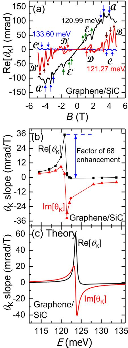
FIG. 1. (a) Magnetic field dependence of  $\text{Re}[\theta_K]$  for multilayer graphene on SiC at 120.99, 121.27, and 133.60 meV. (b) Energy dependence of low-field ( $|B| \leq 1$  T) slope. (c) Calculated Kerr ( $|B| \leq 1$  T) slope for a monolayer graphene on SiC.
