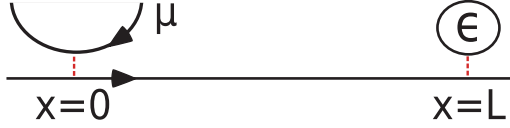
FIG. 5. A QH edge state at the filling factor \nu = (2n + 1)^{-1} , n \in \mathbb{N} , is schematically shown. Electrons are injected at the point x = 0 via the voltage-biased QPC and detected at the point x = L at energies \epsilon with the help of a QD. A measurement setup analogous to the one for integer QH (see Fig. 1) can be utilized.
