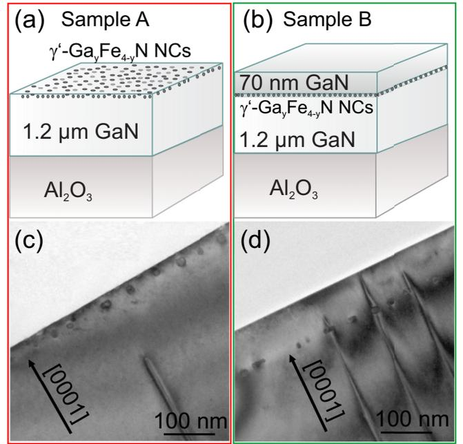
FIG. 1. (a) Schematic representation of sample A, uncapped; (b) schematic representation of sample B, capped with a nominally 70-nm-thick GaN layer. (c) and (d) Cross-section TEM images of samples A and B, respectively, evidencing the spatial distribution of the NCs in a plane perpendicular to the growth direction [0001].
