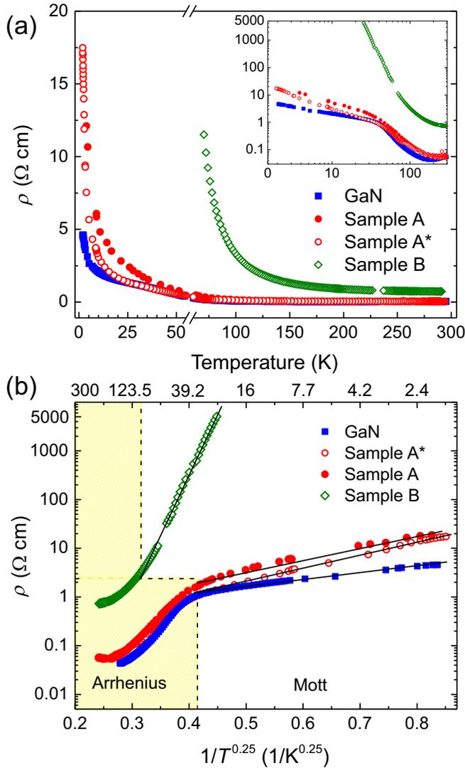
FIG. 5. (a) Resistivity vs temperature for samples A, A\*, and B compared to GaN. Inset: Full scale  $\rho(T)$ . (b) Resistivity vs  $T^{-0.25}$  pointing to a characteristic Mott VRH-type conduction below 40 K for sample A, for sample A\*, and for the GaN reference and below 130 K for sample B. Above these temperatures, an Arrhenius-like behavior is observed.
