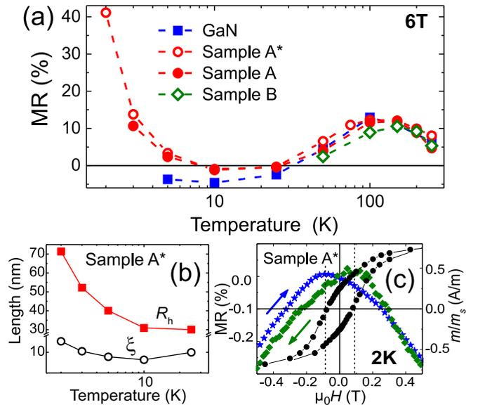
FIG. 7. (a) Comparison of the MR as a function of temperature for samples A, A\*, GaN, and B at 6 T. (b)  $R_h$  and  $\xi$  obtained as a function of temperature for sample A\*. (c) MR and normalized density of magnetic moment as a function of the applied field for sample A\*. The field sweep directions are indicated by arrows.
