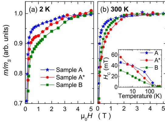
FIG. 3. Normalized magnetic moment of samples A (stars), A\* (dots), and B (squares) (a) at 2 K and (b) at 300 K. Inset in (b): Coercive field strength  $H_c$  vs temperature.
