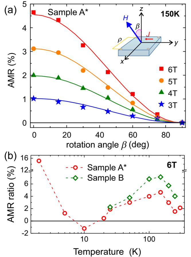
FIG. 8. (a) AMR as a function of the out-of-plane angle  $\beta$  between the magnetic field and the surface normal (symbols) in sample A\* fitted by a  $\cos^2\beta$  function (solid lines). (b) AMR ratio as a function of temperature for samples A\* and B.
