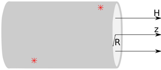
FIG. 4. Thin conducting tube, threaded by a magnetic field H . Impurities (shown as stars) are embedded in the tube. Electrons live on the surface of the cylinder.
