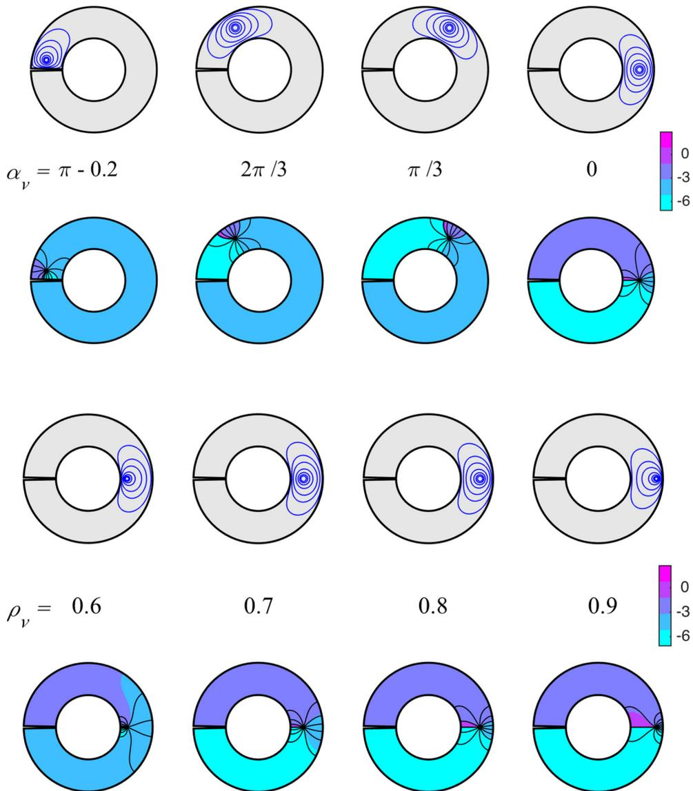
FIG. 3. Contour plots of the stream function  $\sigma_v(x, y)$  and gauge invariant phase  $\phi_v(x, y)$  within the superconducting annulus (inner radius  $\rho_0 = 0.5$ ) when a vortex is present. Upper panel: the position of the vortex is given by  $\rho_v = 0.75$  and decreasing values of  $\alpha_v$ . In the lower panel,  $\alpha_v = 0$  and increasing  $\rho_v$ . The color map has been shifted for visual purposes. Radial coordinates are given in units of  $R$ , i.e.,  $\rho = r/R$ .
