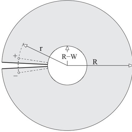
FIG. 1. A superconducting annulus of radius  $R$  and width  $W$  with an edge junction to the left. Ideally, the gap between the upper (+) and lower (-) banks tends to zero, but is oversized for visual purposes. Also sketched is the line contour for integration of the phase variations around the junction.
