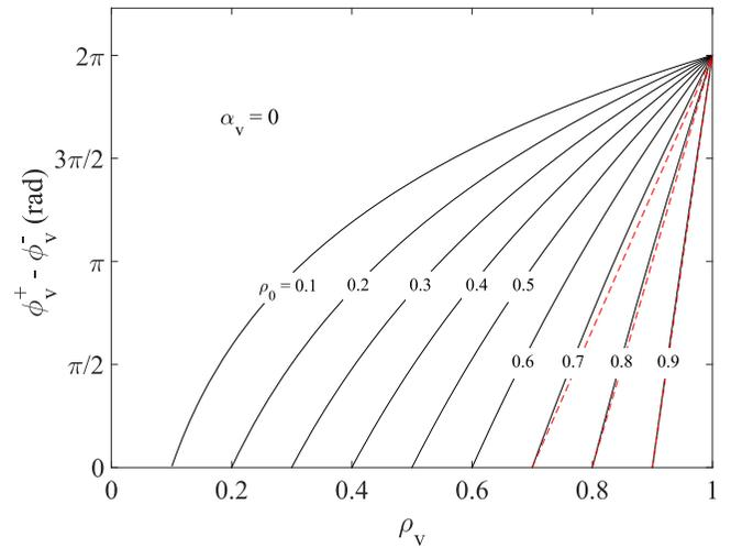
FIG. 5. Averaged phase difference between the two banks of the junction in terms of the radial position of a distant vortex ( $\rho_v$ ) opposite to the aperture ( $\alpha_v = 0$ ). The different lines correspond to superconducting loops of different widths given by the value of the inner radius. For each width, the vortex covers the range  $\rho_0 < \rho_v < 1$ , i.e.,  $R - W < r_v < R$ . The linear approximation [dashed lines corresponding to Eq. (20)] is shown for the thinner loops.
