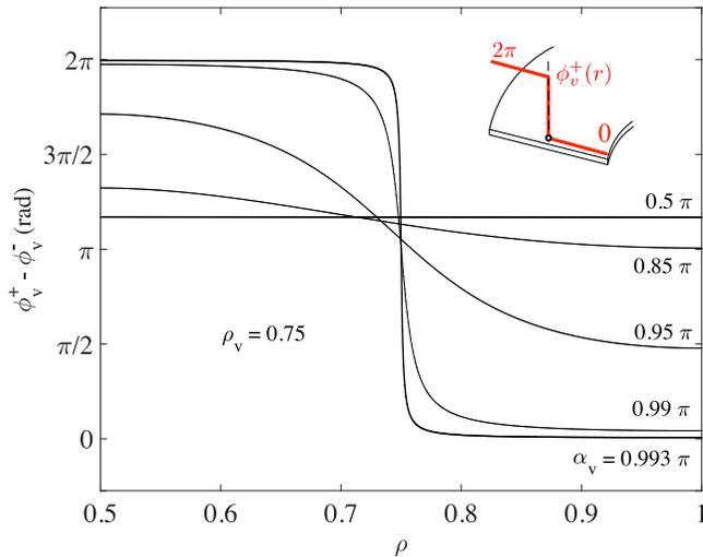
FIG. 4. Gauge invariant phase variation along the banks of the junction for different positions of the vortex given by the coordinates  $(\rho_v, \alpha_v)$ . As in Fig. 3, here  $\rho_0 = 0.5$ . Radial coordinates are relative to the outer radius  $\rho \equiv r/R$ . The inset illustrates the limiting situation in which the vortex is very close to the junction.
