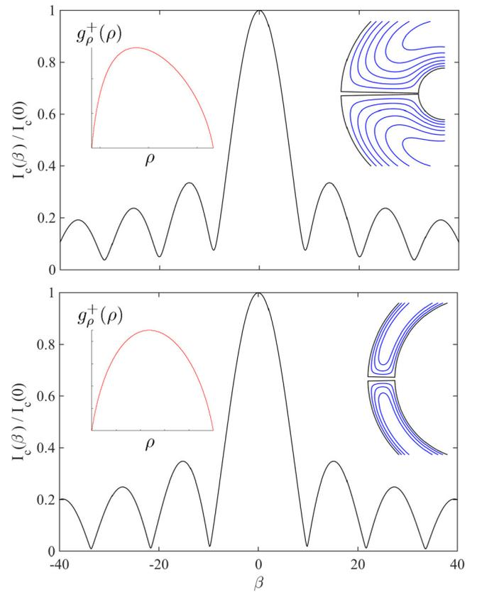
FIG. 6. Critical current pattern in terms of the applied magnetic field with no vortex present. The field is given in dimensionless units  $\beta \equiv 2\pi W^2 B_a / \Phi_0$ . We plot the results for two different loops with respective normalized widths  $W/R = 0.75$  and  $W/R = 0.25$ . The insets to the right show a detail of the streamlines of the current density  $\mathbf{g}$ . To the left, we show the dependence of the radial component  $g_\rho^+$  close to the upper bank of the junction.
