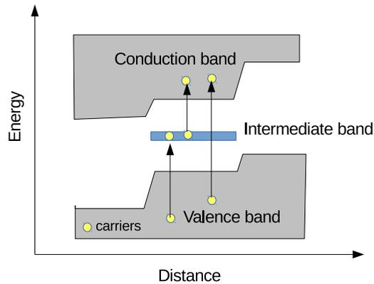
FIG. 1. Schematic of an intermediate band solar cell (adapted from Ref. [4]). Intermediate band states can dramatically improve the efficiency of solar cells by enabling two-photon processes which leads to the increase of photocurrent in a system.
