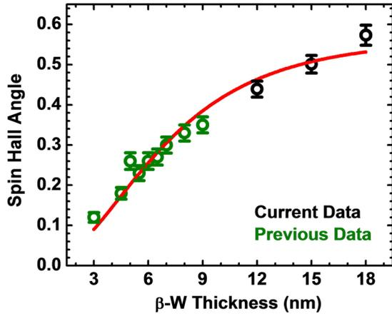
FIG. 4. Spin Hall angle versus  $\beta$ -W thickness, including previous data (green) and current data (black) which has doubled the critical thickness from 9 to 18 nm.
