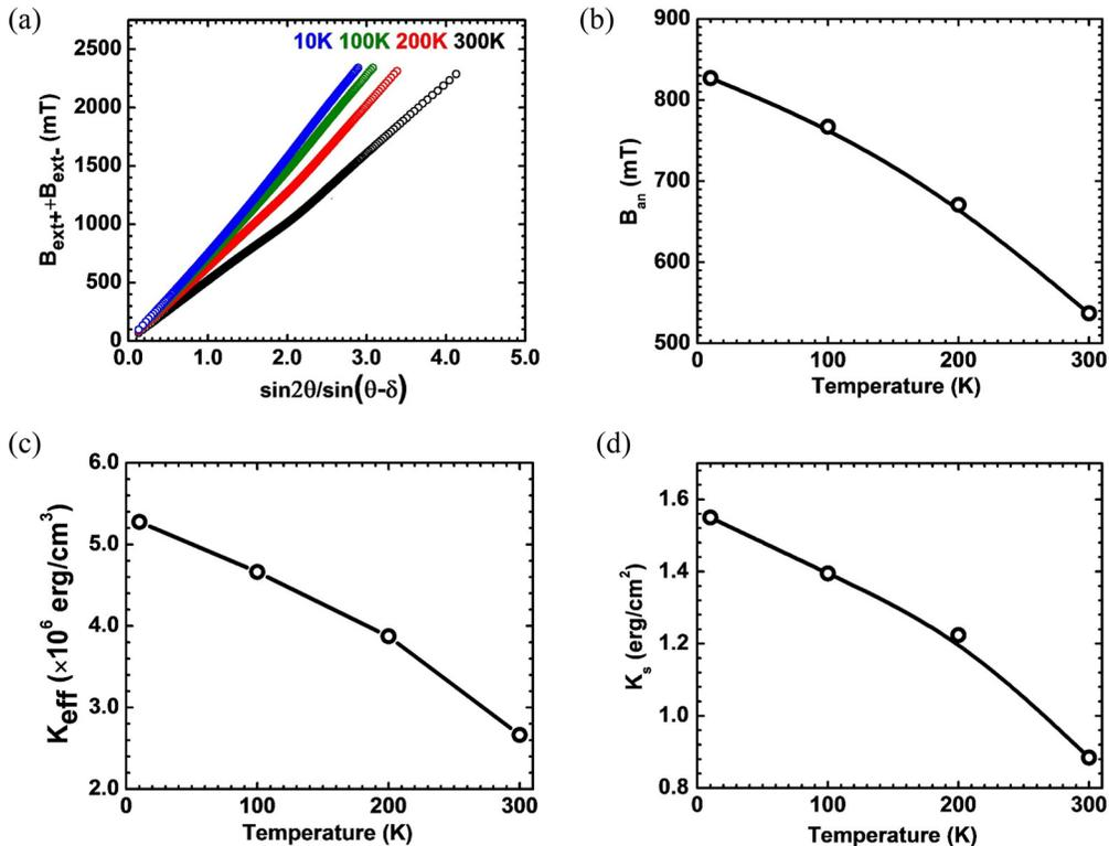
FIG. 5. (a) The value of  $B_{\text{ext}+} + B_{\text{ext}-}$  versus the value of  $\frac{\sin 2\theta}{\sin(\theta-\delta)}$  at different temperatures. (b) Magnetic anisotropy field  $B_{\text{an}}$  versus temperature. (c) Magnetic anisotropy constant  $K_{\text{eff}}$  versus temperature. (d) Magnetic surface anisotropy constant  $K_s$  versus temperature.
