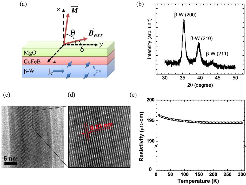
FIG. 1. (a) A schematic view of the sample under transport measurement with  $y$ -axis charge current  $J_c$  under the external field  $\vec{B}_{ext}$ .  $\vec{M}$  is the magnetization vector of the CoFeB layer with PMA. (b)  $\theta$ - $2\theta$  X-ray diffraction pattern confirming  $\beta$ -W phase. (c) and (d) HRTEM image of the cross section of the multilayer sample. The atomic interplanar spacing is 2.3 Å. (e) Resistivity of the  $\beta$ -W layer versus temperature.
