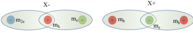
FIG. 4. Illustration of negative (left) and positive (right) trions in tungsten-based TMDs. Because of the repulsion between charges with the same sign and the resulting larger separation between them, we can view the trion as comprised of two electron-hole pairs, where each contributes about one-half to the trion binding energy. The difference in binding energy of the \{m_{2e}, m_h\} pair in X_- and the \{m_e, m_h\} pair in X_+ leads to the relatively large difference between the binding energies of negative and positive trions, as written in Eq. (D6).
