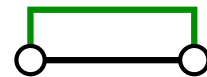
FIG. 2. The lowest-order diagram for the kernel \Sigma_a(E) . Here, the circles represent the bare vertices G , the black line connecting the vertices is the local propagator and the green line denotes the bath contraction.
