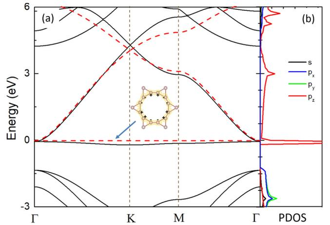
FIG. 2. (a) Band structure of kagome graphene, where the solid and dashed lines are the calculated results of DFT and the tight-binding model in Eq. (1), respectively. Inset shows the wave function for a localized state in the flat band. (b) Partial density of states (PDOS) of kagome graphene.
