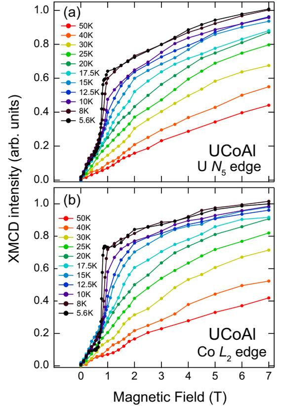
FIG. 2.  $H$  dependence of the XMCD intensity (M-H curve) at several  $T$ s. (a) The M-H curve at the U  $N_5$  edge ( $h\nu = 735.0$  eV) and (b) that at the Co  $L_2$  edge ( $h\nu = 794.5$  eV). These photon-energy positions are indicated by the arrows, as shown in Fig. 1(b). The M-H curves are normalized so that the XMCD intensity at  $T = 5.6$  K and  $H = 7$  T becomes 1.
