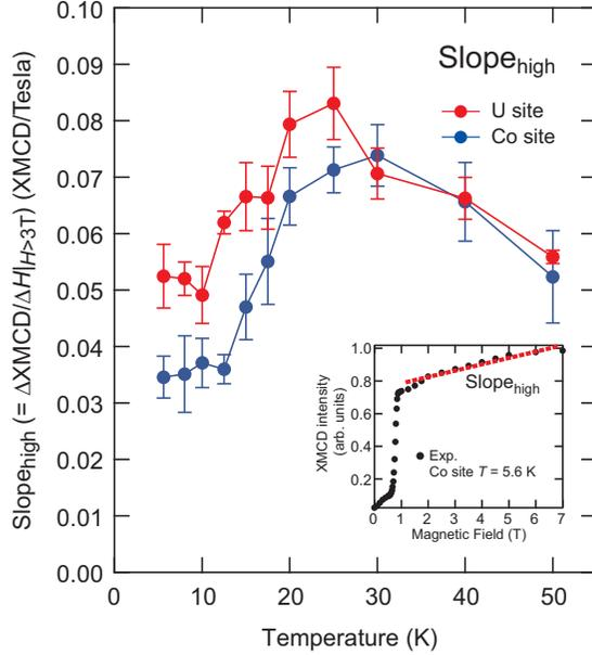
FIG. 4.  $T$  dependence of the slope of the element-specific M-H curve in the high magnetic field region ( $S_{\text{high}}$ ), obtained by fitting the M-H curve above  $H = 3$  T with a straight line. The scale of the vertical axis is the same as that in Figs. 2(a) and 2(b). The inset shows an example of the  $S_{\text{high}}$  at the Co site at 5.6 K.
