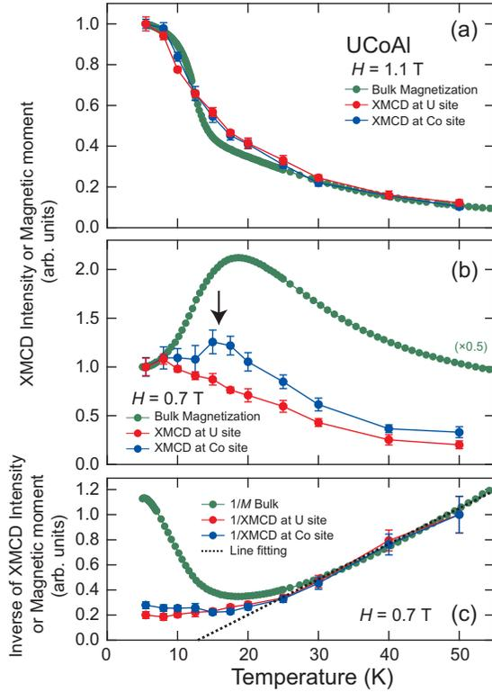
FIG. 6. Comparison between the element-specific and bulk M-T curves [8]. (a) At  $H = 1.1$  T above  $H_M$ . (b) At  $H = 0.7$  T below  $H_M$ . The profiles in (a) and (b) are normalized at  $T = 5.6$  K. The M-T curve of the bulk magnetization at  $H = 0.7$  T is multiplied by 0.5. (c) Inverse plots of the M-T curves at  $H = 0.7$  T displayed in (b), which is normalized at  $T = 50$  K for easy comparison.
