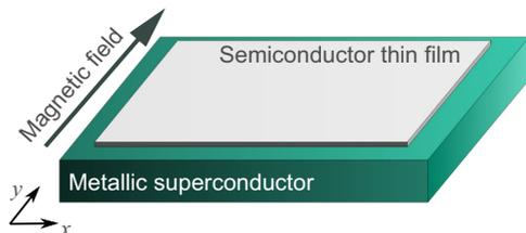
FIG. 1. Schematic image of a Dresselhaus [110] superconductor.
