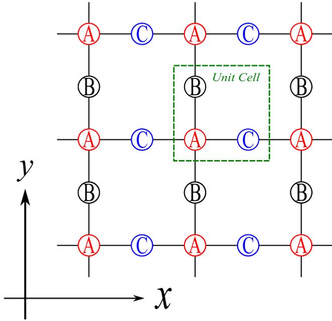
FIG. 1. Two-dimensional Lieb lattice. Its unit cell, which contains three atoms (A, B, C), is shown as the dashed line. The corresponding density of states for the noninteracting case can be found, for example, in Refs. [25] and [26].
