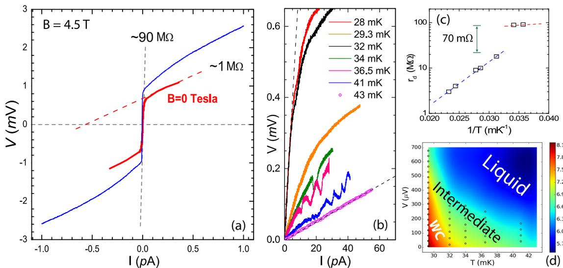
FIG. 4. (a) dc IV at  $T = 28 \text{ mK}$ . (b) IVs obtained at different  $T$ . (c)  $T$  dependence of  $r_d(T)|_{V \rightarrow 0}$  on semilogarithmic scales. (d) Colored contour phase diagram based on  $\log_{10} r_d(T)$  values. Dashed lines are guides.
