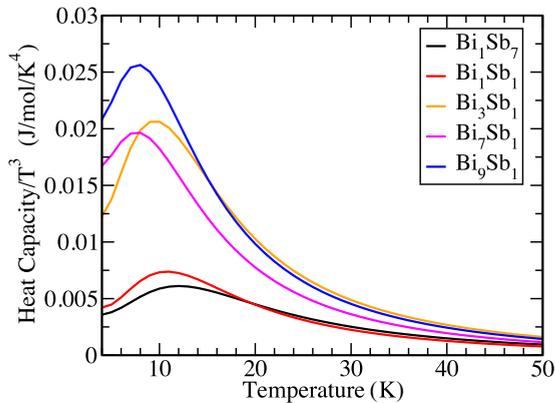
FIG. 6.  $C(T)/T^3$  vs temperature  $T$  data for Bi-Sb binaries.
