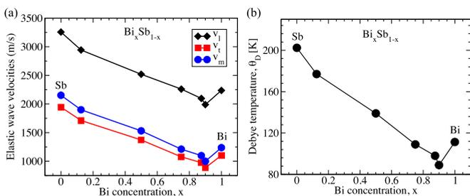
FIG. 5. (a) Elastic wave velocities and (b) Debye temperature ( $\Theta_D$ ) of Bi-Sb binaries calculated with SOC.
