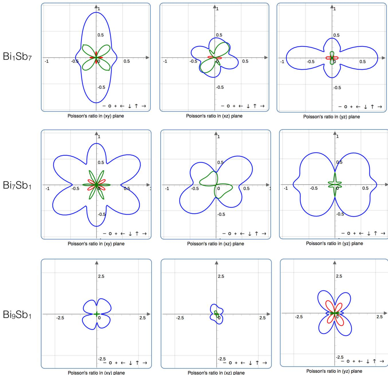
FIG. 3. Top, middle, and bottom panels represent the calculated Poisson's ratio of  $\text{Bi}_1\text{Sb}_7$ ,  $\text{Bi}_7\text{Sb}_1$ , and  $\text{Bi}_9\text{Sb}_1$  binaries, respectively. All plots were generated using the ELATE software [61]. Green (red) corresponds to the positive (negative) values of  $\nu$  (see text for details).
