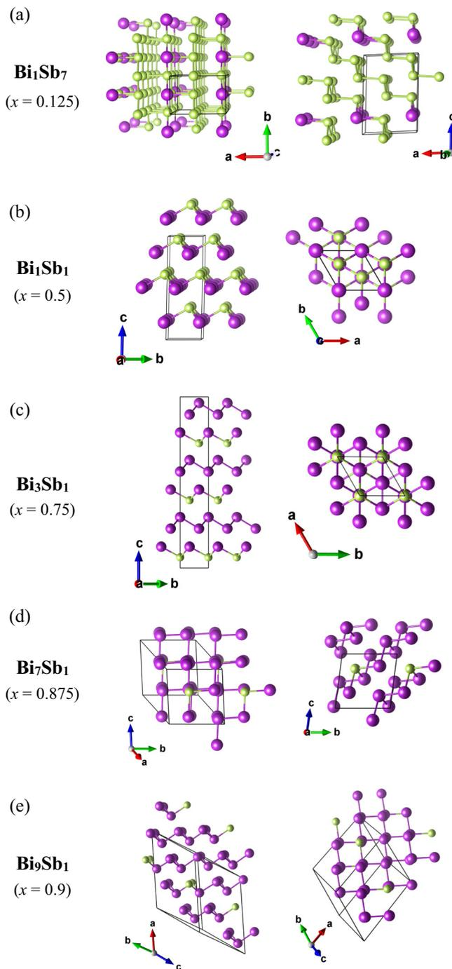
FIG. 1. The crystal structure of Bi-Sb binaries located on the Bi-Sb phase diagram [12]. Bi atoms are shown in purple, while Sb atoms are shown in green. Each crystal structure is shown from two different lattice orientations. The cutoff length for bonds was defined as 3.10 Å in Sb-rich compositions and 3.20 Å in Bi-rich compositions.
