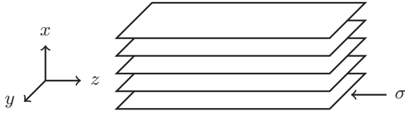
FIG. 1. Geometry of the plasmonic crystal. The layered structure is periodic in the x direction and consists of planar 2D metallic sheets with isotropic conductivity \sigma .
