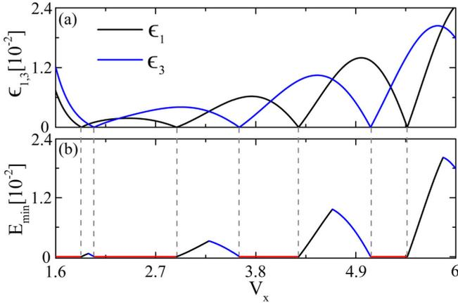
FIG. 3. (a) Oscillatory dependence of energy splitting on Zeeman energy in different nanowires. (b) Smallest value of lowest-energy excitations within  $\Phi \in [0, \Phi_0]$  at different  $V_x$ . Red lines show the regime where gapless excitations are available. We use  $\{\Gamma_0, \Gamma_l\} = \{3, 3\}$  and other parameters are the same as Fig. 2.
