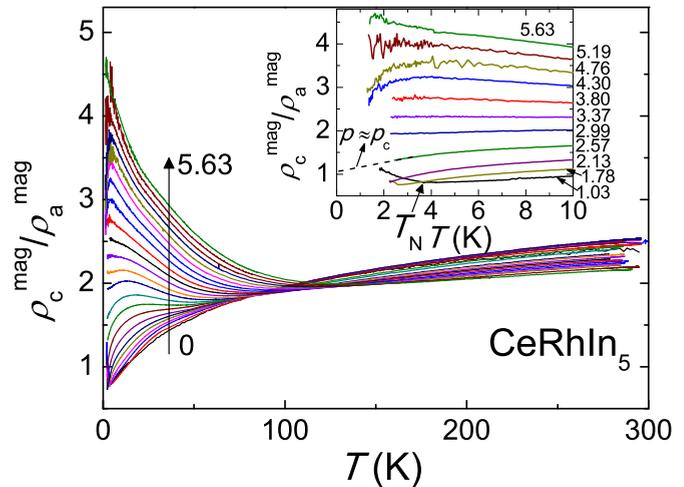
FIG. 2. Temperature dependencies of the magnetic resistivity anisotropy under pressures up to 5.63 GPa. The inset shows a zoom of the data below 10 K at selected pressures. The dashed line is an extrapolation of the curve at  $p \approx p_c$  to zero temperature.
