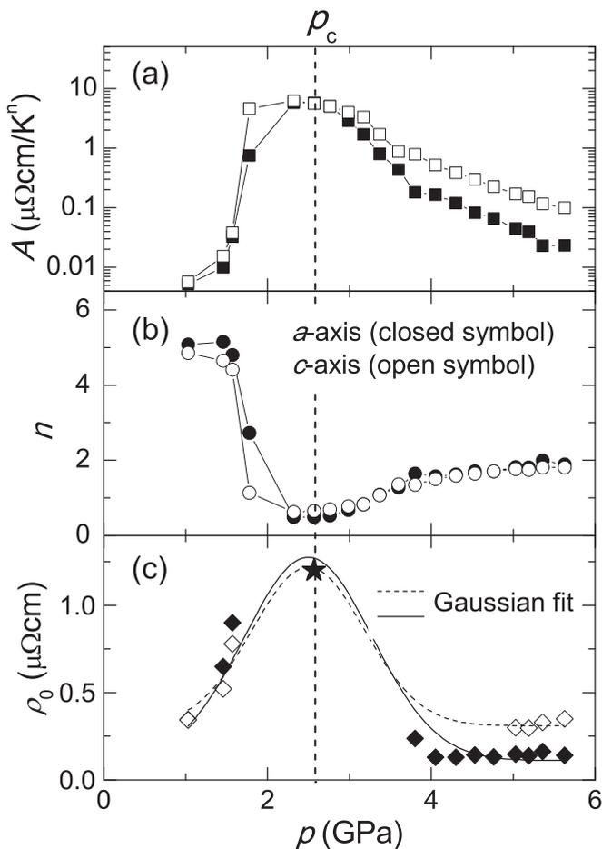
FIG. 3. (a)–(c) The pressure dependencies of the coefficient  $A$ , temperature exponent  $n$ , and residual resistivity  $\rho_0$ , respectively, obtained by fitting with the power law  $\rho(T) = \rho_0 + AT^n$  to the  $a$ - (closed symbol) and  $c$ -axis (open symbol) resistivity data at low temperature. Note that the high-field value at 2.57 GPa in (c) is taken from Ref. [12] and assumed to be isotropic.
