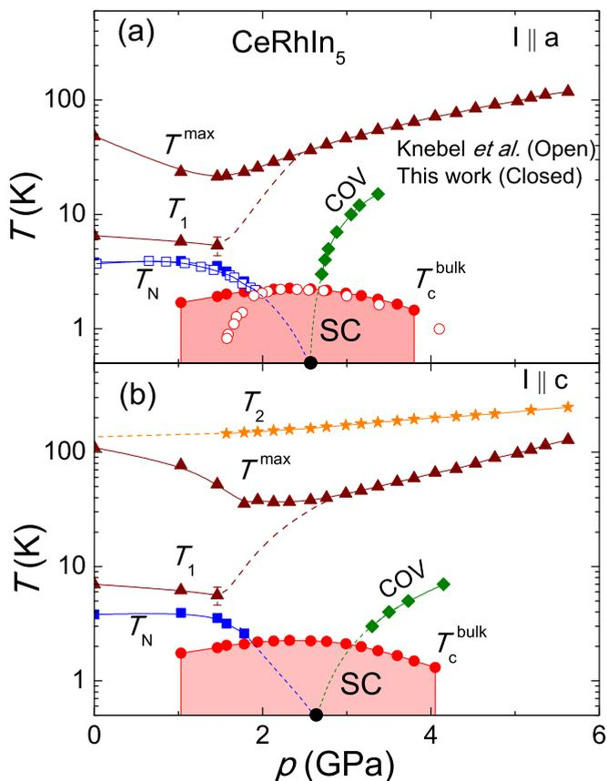
FIG. 5. Pressure-temperature phase diagram of  $\text{CeRhIn}_5$  along the (a)  $a$  and (b)  $c$  axes, including the characteristic temperatures  $T_1$ ,  $T_2$ , and  $T^{\text{max}}$ . For comparison, data from Ref. [12] are also included in (a).
